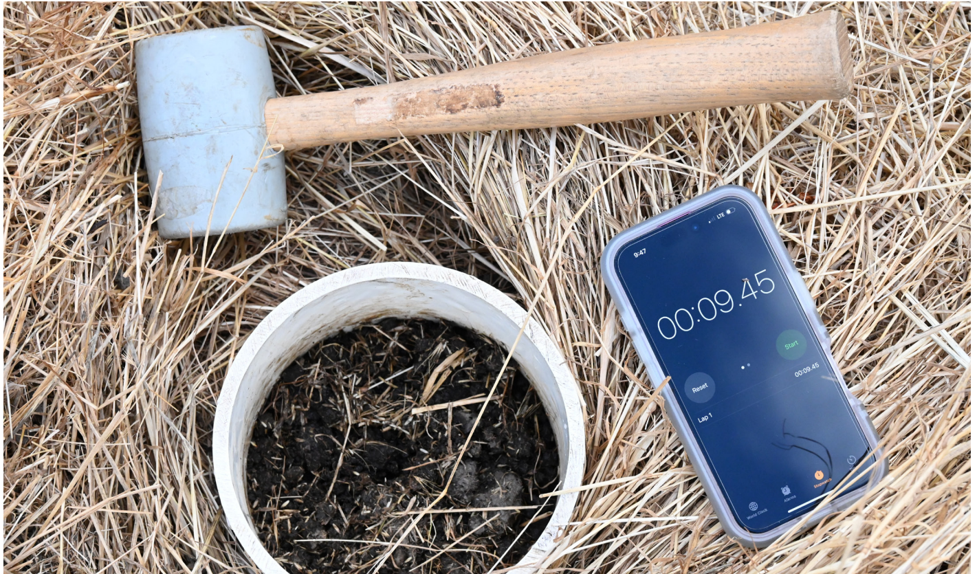
What you need for a water infiltration test
